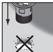
Please ensure that there is no grime on the edge of the hole when installing the drain cup. Local voltage peaks resulting from contact with hard materials, such as metal, can quickly lead to breakage.
