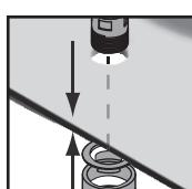
To prevent stress cracks in the tap and drain area, we recommend using appropriate sealing material (rubber or plastic inserts) or permanently elastic sealing compound (installation kit for hot and cold water). Ensure that the affixing material is suitable for use on the washbasin.
